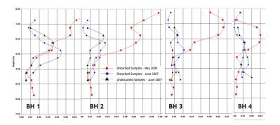
Soil tests undertaken in May 2006 (left) reveal the presence of a persistent moisture deficit carried over from the previous year.
